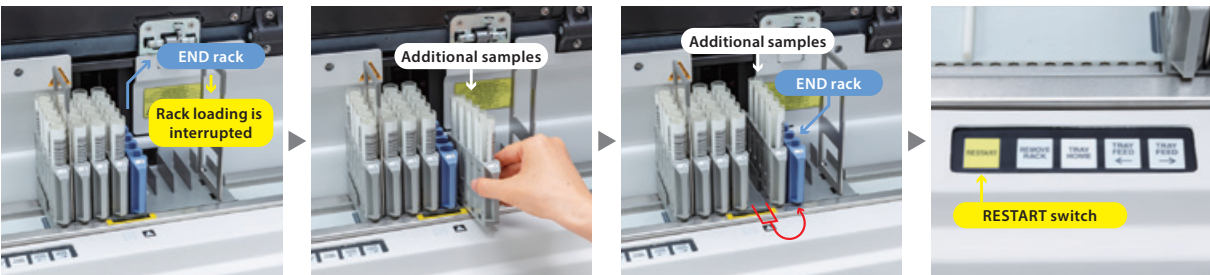
Rack loading is interrupted when the system detects the END rack.
